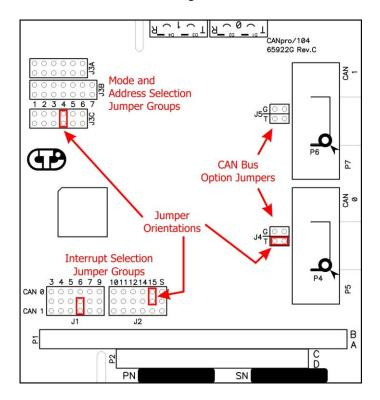
The jumper positions are numbered on the PCB (and are shown in the above drawing). **J1 and J2** are **Interrupt Selection** jumpers, and the numbers (3, 4, 5, 6, 7, 9, 10, 11, 12, 14 and 15) refer to the actual interrupt number being selected. **J3A, J3B and J3C** positions are numbered sequentially from left to right. J3A and J3C have 6 positions, J3B has 7 positions. **J4 and J5** positions are labeled "T" and "G".
